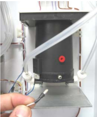
Banana Plug – Be sure to cover to prevent shorting.
