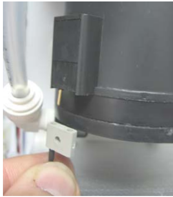
Block Connector. Gently pull away from sensor pin.
