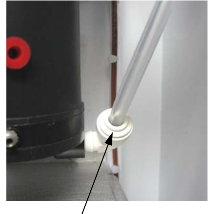
Tube Fitting inner collar. Press in while pulling out on the tubing.
